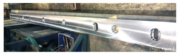
**Figure 3.** For machine components working under the most demanding conditions, laser hardening improves lifetime. SSAB is using laser hardened Toolox® 44 for cutting Hardox® and Strenx® steel plates. The shearing blades are seen in figure 3. A high hardness and strength are due to the thickness and high hardness of the products.
